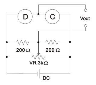
For fixed and variable resisters in this circuit = Metal covered resistors are preferable.
