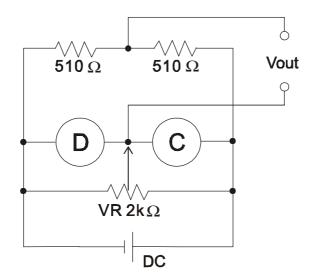
For fixed and variable resisters in this circuit = Metal covered resistors are preferable. Especially the resistor of  $510\Omega$  should be of high quality with a tolerance +/- 1% or less. 9. Typical gas sensitivity characteristics
